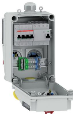
2. Strip the cable such that the sheath reaches about 1 cm wide through the cable gland in the distributor. Remove the insulation from the cable cores.
