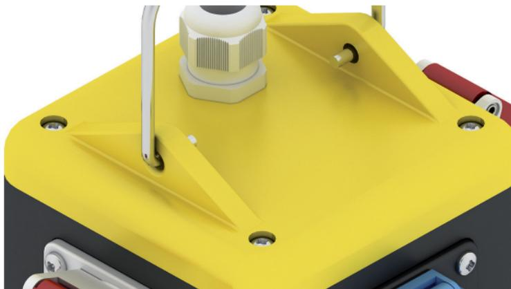
2. Strip the cable such that the sheath reaches about 1 cm wide through the cable gland in the distributor. Remove the insulation from the cable cores.
