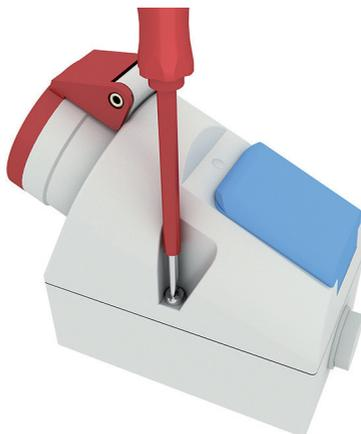
3. Loosen the screws on the contacts of the connection terminal and the screws (5) on the contacts of the three-phase outlet to which the cable is connected, and pull the individual conductors out of the terminals.
