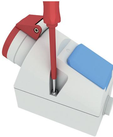
5. For variants without wiring: Create the necessary connections within the surface-mounting socket outlet according to one of the three possible connection options and test them. Tighten the screws on the connection terminals (7) with a torque of at least 1.2 Nm.
